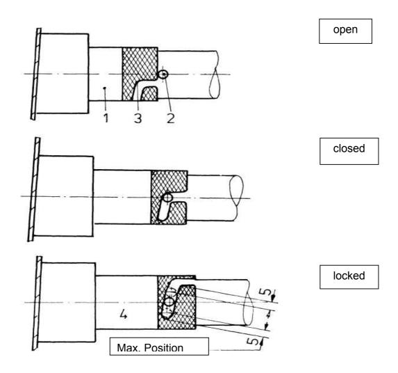
After connecting the quick lock couplings make a visual check that the collar is extended forward over the bearing far enough for the safety pin to engage.
