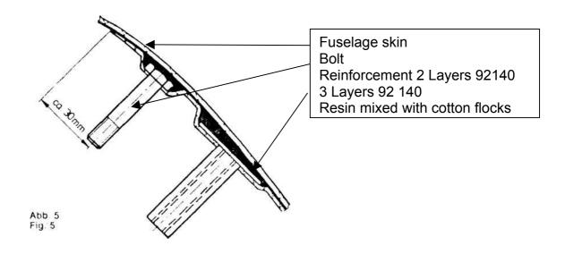
The fitting shall be made as shown in the drawing so as to take the weight of the additional equipment. Under loads of up to 10g no piece of equipment must come loose from it's support. Following installation of additional equipment, a weight and balance report shall be compiled to ascertain that the C of G is within the permitted limits.
